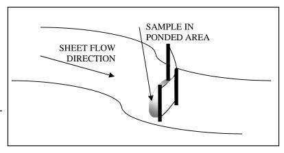
(e.g. 2-3 feet of silt fence installed in a U-shaped fashion; or an asphalt berm on paved areas). These areas should be stabilized prior to sampling with rolled erosion control product or sod to avoid increased turbidity at the sampling point. If necessary, use a clean, shallow scoop (e.g. dustpan) to collect the sample and deposit it in a sample bottle.
